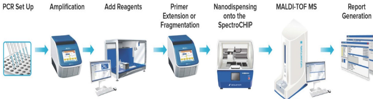
Figure 7: Workflow for validation of whole genome sequencing findings using Yale cohort of tissue. DNA from formalin-fixed, paraffin embedded tumor tissue and also genomic controls will be amplified, have primer extension, mass spectroscopy detection, and analysis. Germline and somatic, coding and non-coding variants will be validated with a large Yale patient cohort.
