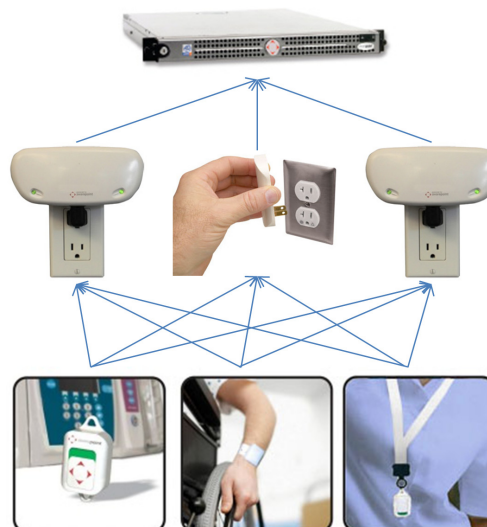
Figure 1: A demonstration of the real-time location system in hospitals. At the bottom layer, the moving objects (medical devices, patients, doctors, etc.) are attached with sensor tags, which send signals to the sensor receivers. The sensor receivers at the middle layer transmit the signal data to the network bridges. At the top layer, network bridges connected with data/application servers will collect the signal data and the data/application servers will calculate locations of the tracked objects.
